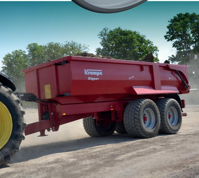
**Profi-Line+** is designed to cope with heavier loads and high speeds of up to 80 km/h. Available on request for speeds up to 100 km/h.
